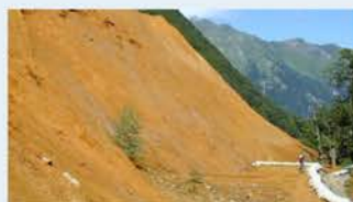
▲ Dumps of flotation residue from tungsten mining (Salau, France) still contain a high value in tungsten [2].
