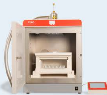
◀ Microwave-assisted fusion is developed in TARANTULA to increase recovery of W, Nb and Ta [3].
