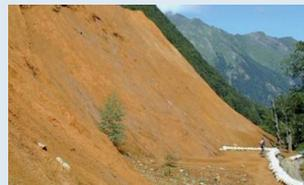
▲ Dumps of flotation residue from tungsten mining (Salau, France) still contain a high value in tungsten [2].
