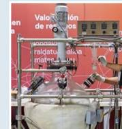
▲ Deep Eutectic Solvents (DES) systems for leaching followed by liquid/liquid extraction technologies and electrodeposition are used in TARANTULA to increase the recovery of W, Nb and Ta
