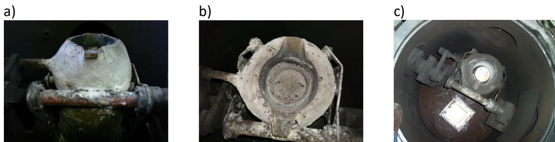
Figure 23. Melting crucible: a) general view; b) crucible in dump position; c) crucible with electrolytic iron and ingot mould inside the vacuum chamber.
