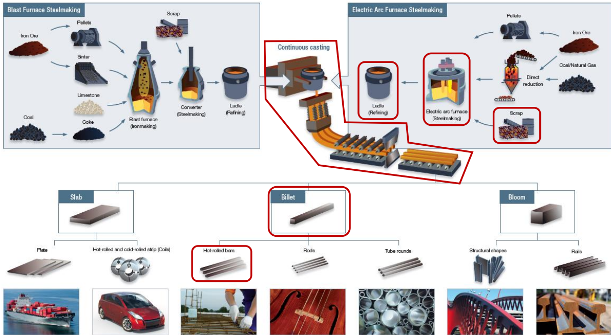
Figure 14. Steelmaking routes based on CC and types of steel products.
